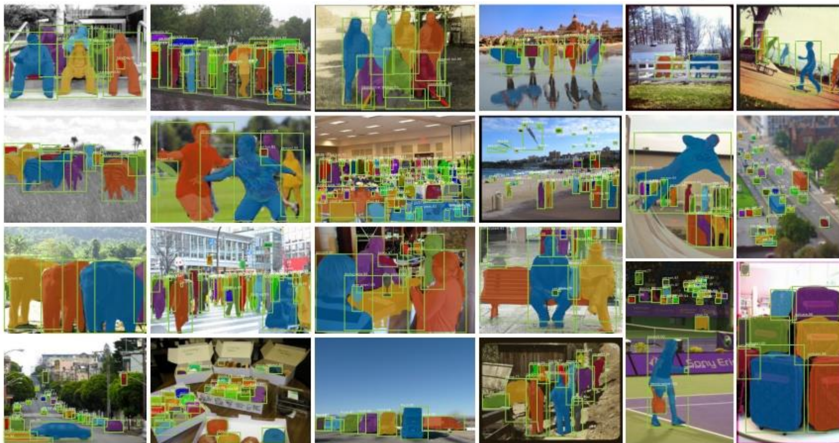
Figure 4. More results of Mask R-CNN on COCO test images, using ResNet-101-FPN and running at 5 fps, with 35.7 mask AP (Table 1).
